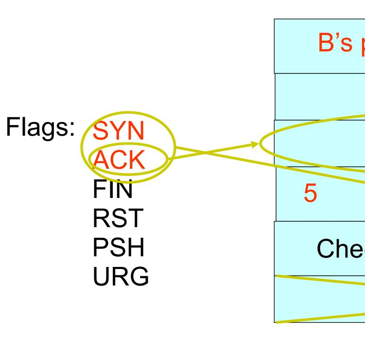
B tells A it accepts, and is ready to hear the next byte... ... upon receiving this packet, A can start sending data
